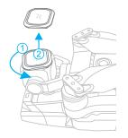
取下原装镜片 Remove the original lens
