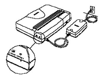
When the battery is fully charged, the CHARGE light turns off.
