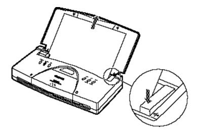
☐ If the leading edge of the jammed sheet is coming out of the paper exit slot, pull the paper out carefully from the paper exit slot.
