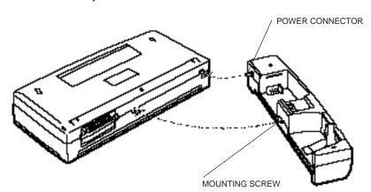
5. Fasten the battery case to the printer by turning the thumbwheel to the right (toward the mark).
